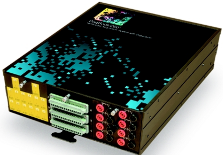
The DaqBook/260 data acquisition system offers easy expansion and your choice of connectivity (shown here with optional DBK605, DBK606, and DBK604 termination panels)
